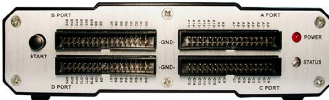
Fig. 1-10: Rear view of the Zeroplus Logic Analyzer LAP-B Series.
